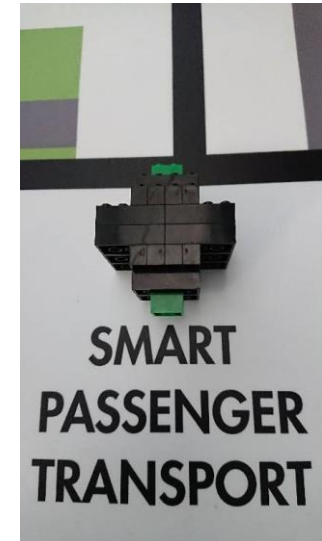
A Green (2x2) LEGO brick is added on to the bottom of the battery to place it on the black line “T” of the start area
